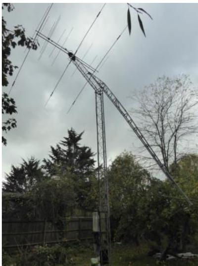
The combination of the IC7300 and TA33 was very effective with a total of 171, 94 and 77 QSOs were made on 20, 15 and 10m respectively. The other 3 bands (160, 80 and 40m) were also in use using an IC706 MK2G with either a random length wire or a 40m inverted 'V' dipole.
