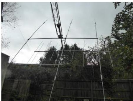
The optimal resonance for each band depends on various element lengths but those chosen were not ideal for the 14, 21 and 28MHz bands. The new IC7300 has an internal ATU (AMU) and this was very successful in 'fine
